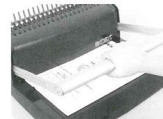
(Fig. 4) Pull the Punching handle all the way down until it stops to punch completely through
