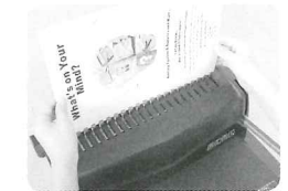
(Fig. 6) Load punched sheets directly onto the opened comb
