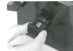
(Fig. 2) Punching preparation: Pull the Punching margin control from 2mm to 5mm
