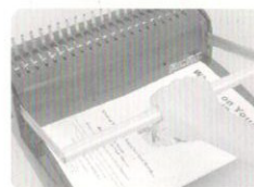
(Fig. 4) Pull the Handle all the way down until it stops to punch completely through
