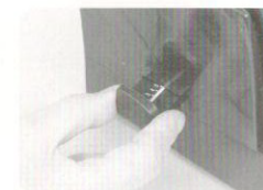
(Fig. 2) Punching preparation: Pull the Punching margin control from 2mm to 5mm
